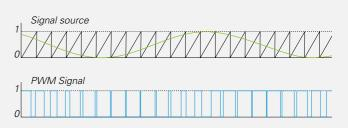
A sinusoidal curve (=) can be converted into a PWM signal (=), for example, by comparing it with a saw-tooth-shaped signal (=). For each PWM pulse, the sawtooth ramp runs through the entire value range. This means that on inert loads such as motors, the PWM voltage curve acts like a sinusoidal voltage.
